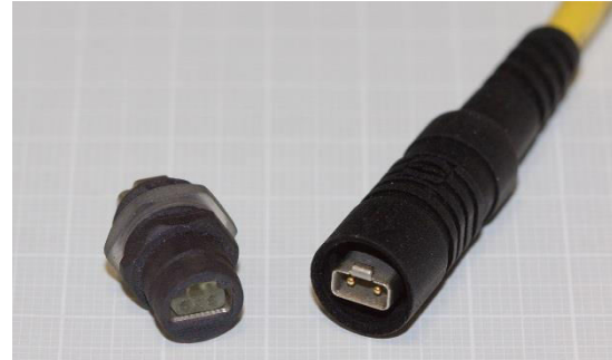
Prototype M8 style, plug overmolded and straight PCB THR jack with housing
